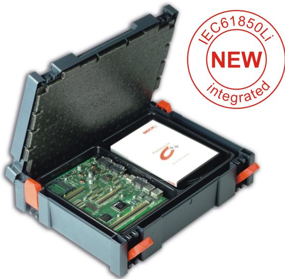
The IPC@CHIP® DK61 Development Kit is a complete development system for the new IPC@CHIP® SC123 and SC143 Embedded Controllers.
