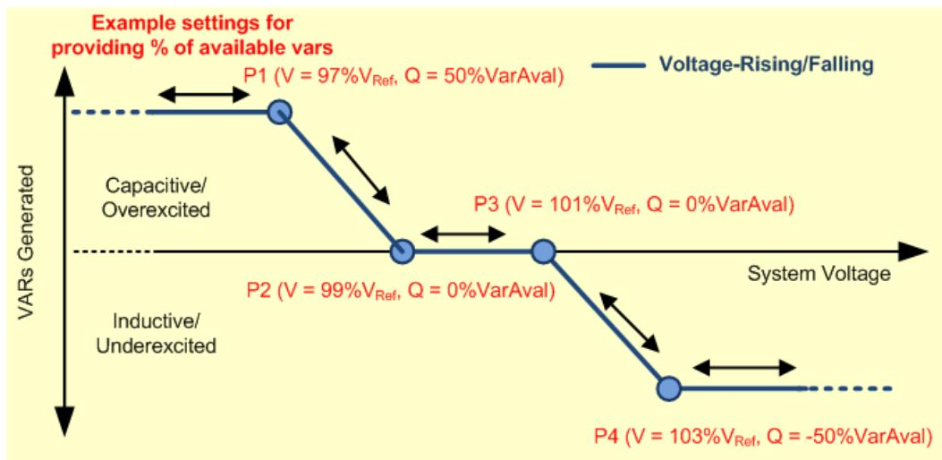
The information needed for this application is defined in corresponding Logical Nodes of IEC 61850-90-7 and IEC 61850-7-4. From an implementation point of view the standard just provides an external view of the inverter internal information and information exchange (**for the inverter functions, e.g., volt-var control**). It could be assumed that the functions are **already implemented in the existing inverter controller**. Possible implementation architectures are:
