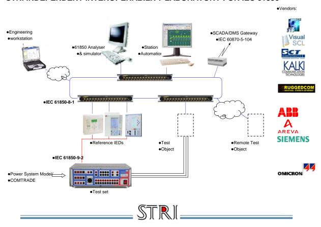
A complete substation can be modeled using state-of-the art IEDs from ABB, Areva and Siemens, switches from RuggedCom and test sets from Omicron and Doble. Additional IEDs, switches, gate ways and test sets from other manufacturers can be added. Vendor specific as well as third party software is used for IEC 61850 engineering and configuration. The interoperability verification will consequently cover both IEDs, switches, software and test sets.
