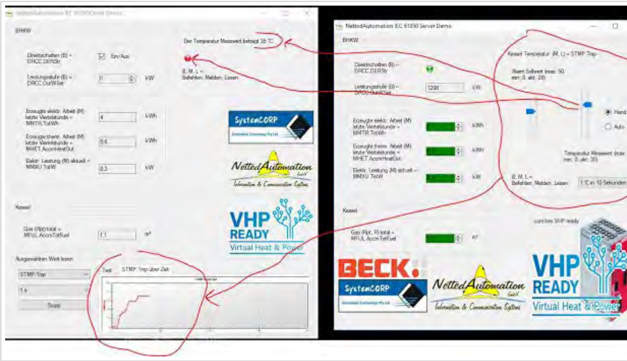
A SCL DataTypeTemplate for a temperature measurement "STMP_0" could be bound to a graphical representation.
