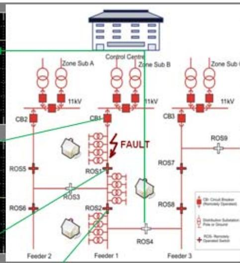
**FLISR scenario: fault is on CB1 section, supply restored on ROS1 and ROS2 sections**
